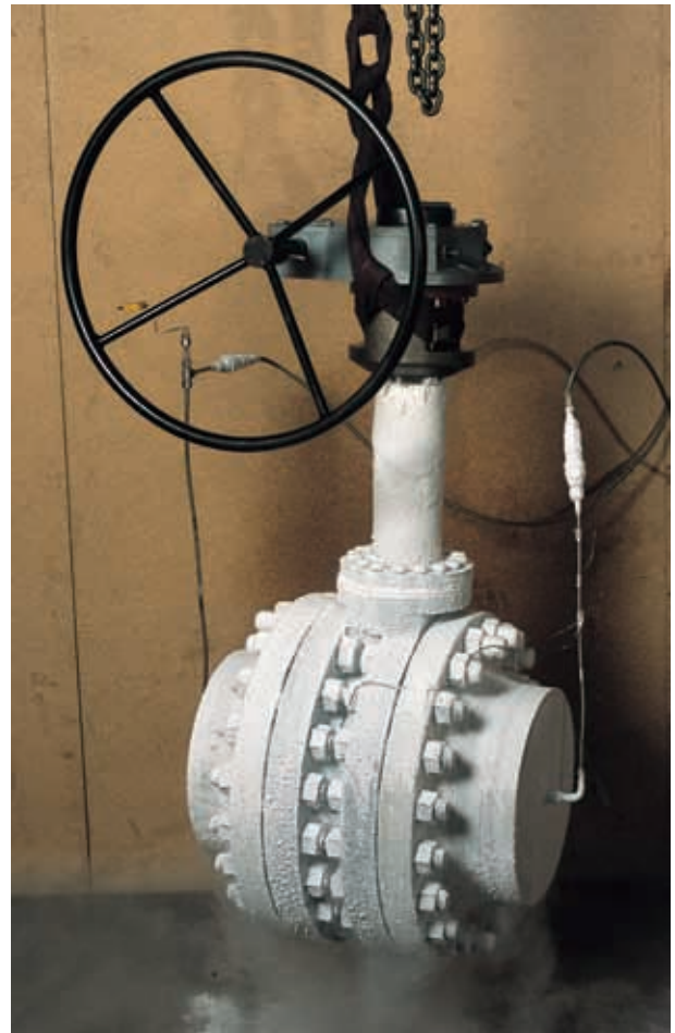
Cryseal valve undergoing low temperature liquid nitrogen test (photos courtesy Valve Testing Centre, Leeds University)
