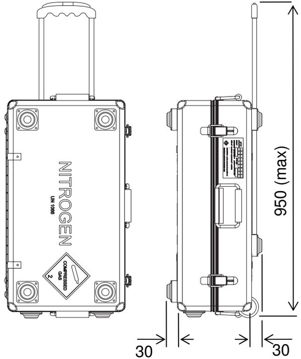
For ease of transport we can now supply the PCU fitted with wheels and an extendable handle. These can be fitted to any configuration of PCU and a retrofit kit is available. Both the wheels and the handle are selected from proven applications and are both rugged and practical.
